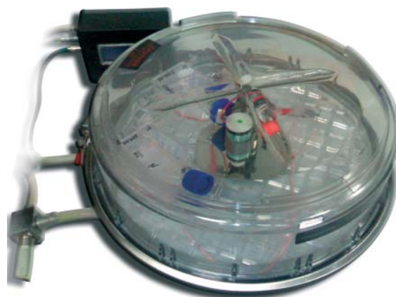
Fig. 1. Chamber for exposure of cell cultures under conditions of modified gaseous medium.
